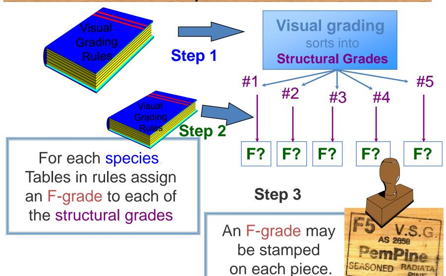
The output of a visual grading process is a **structural grading** - Grades are structural No. 1 to structural No. 5. Within a species, it can be said that structural No. 1 should perform better than structural No 4. Each species has an F-grade assigned for each structural grade number. For example:
